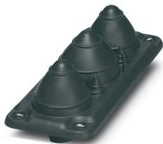
Cable feed-through plates, no. of conductors: 7, external cable diameter: 1x 30 mm ... 60 mm, 4x 10 mm ... 14 mm, 2x 24 mm ... 54 mm, material: galvanized sheet steel (Core), material: TPE-SEBS (external material), color: black, length: 222 mm, width: 92 mm, height: 43 mm
