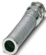
Cable gland, material for screw connection: Brass, nickel-plated, application: Standard, external cable diameter 13 mm ... 21 mm, shielding: no, connecting thread: M32 x 1.5, color: silver-colored, with bend protection sleeve, with O-ring
