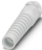
Cable gland, material for screw connection: PA, application: Standard, external cable diameter 3 mm ... 7 mm, shielding: no, connecting thread: M12 x 1.5, color: lightgray RAL 7035, with bend protection sleeve
