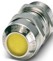
Cable gland, material for screw connection: Brass, nickel-plated, application: Ex, external cable diameter 10 mm ... 17 mm, shielding: no, connecting thread: M25 x 1.5, color: silver-colored, with O-ring
