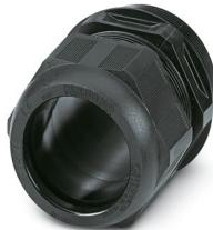
Cable gland, material for screw connection: PA, application: Ex, external cable diameter 34 mm .. 48 mm, shielding: no, connecting thread: M63 x 1.5, color: jet black, with flat gasket
