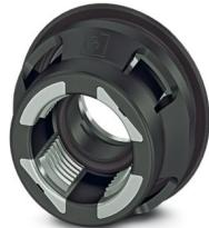
M12 housing screw connection with tolerance-compensating function, for straight, THR solderable M12 socket contact inserts. Suitable for 3.1 mm ... 3.9 mm thick front plates.
