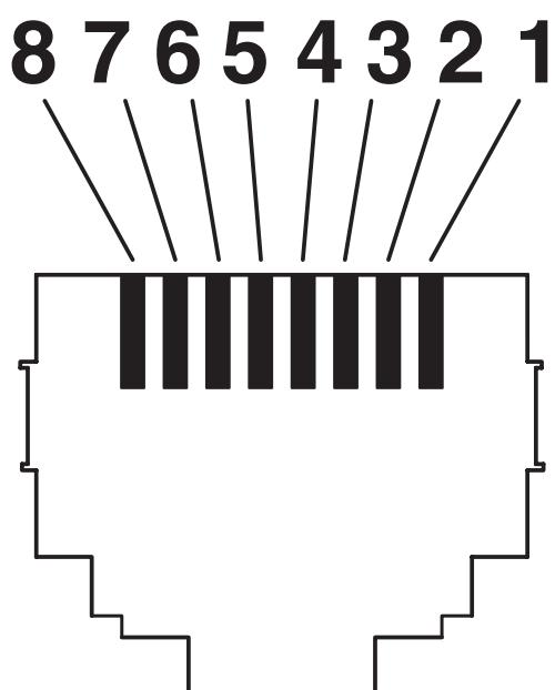
Connector pin assignment plug RJ45
