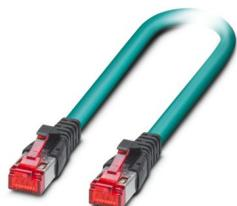
Patch cable, degree of protection: IP20, cable length: 2 m, number of positions: 8, 10 Gbps, CAT6<sub>A</sub>, connection method: Pierce connection, Ethernet, 2x2xAWG26/7, S/FTP, water blue RAL 5021
