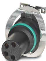
Contact carrier, 4-position, Socket, straight, M8, A-coding, SMD reflow, this item is expected to be lead-free from Q1 2027 in accordance with RoHS II without exception 6c (Pb < 0.1%), a lead-free alternative is possible on request in advance
