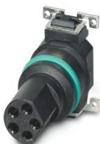
Contact carrier, Universal, 5-position, Socket, straight, M8, B-coding, SMD reflow, this item is expected to be lead-free from Q1 2027 in accordance with RoHS II without exception 6c (Pb < 0.1%), a lead-free alternative is possible on request in advance
