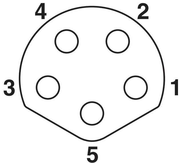
Pin assignment of M8 socket, 5-pos., B-coded
