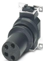
Contact carrier, 4-position, Socket, straight, M8, A-coding, SMD reflow, this item is expected to be lead-free from Q1 2027 in accordance with RoHS II without exception 6c (Pb < 0.1%), a lead-free alternative is possible on request in advance
