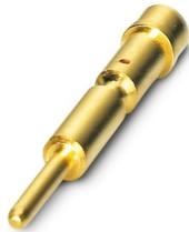
Crimp contact, series: VARIOCON, Pin, turned, contact diameter: 1 mm, connection cross section: 0.14 mm<sup>2</sup> ... 0.5 mm<sup>2</sup>, AWG 26...20, contact material: Cu, this item is expected to be lead-free from Q1 2026 in accordance with RoHS II without exception 6c (Pb < 0.1%), a lead-free alternative is possible on request in advance
