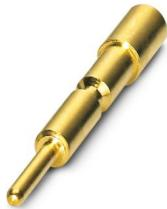
Crimp contact, series: VARIOCON, Pin, turned, contact diameter: 1 mm, connection cross section: 0.14 mm<sup>2</sup> ... 1 mm<sup>2</sup>, AWG 26...18, contact material: Cu, this item is expected to be lead-free from Q4 2025 in accordance with RoHS II without exception 6c (Pb < 0.1%), a lead-free alternative is possible on request in advance
