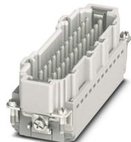
Contact insert, number of positions: 24+PE, size: B24, number of connections per position: 1, Pin, Push-in connection, 500 V, 16 A, 0.14 mm<sup>2</sup> ... 2.5 mm<sup>2</sup>, application: Power
