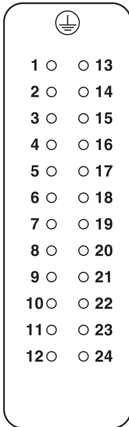
Pin assignment, connection side, socket
