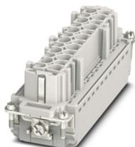
Contact insert, number of positions: 24+PE, size: B24, number of connections per position: 1, Socket, Push-in connection, 500 V, 16 A, 0.14 mm<sup>2</sup> ... 2.5 mm<sup>2</sup>, application: Power
