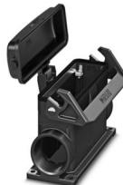
Surface mounting housing B24, with single locking latch, material: PA 6.6-FR, protective cover material: PC, cable outlets: 2, lateral, 2x M40, height: 84 mm, cable gland: none, protective cover: yes, Standard
