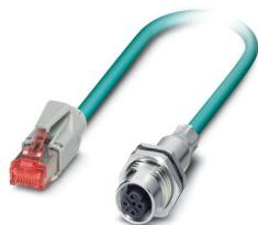
Assembled Ethernet cable, CAT5e, shielded, 2-pair, 26 AWG stranded (7-wire), RAL 5021 (water blue), M12 flush-type socket, rear/screw mounting with SPEEDCON to RJ45 plug/IP20, line, length: 0.3 m
