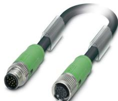
Sensor/actuator cable, 17-pos., PUR/PVC, RAL 9005 (black), shielded, straight M12 SPEEDCON male plug (A-coded) to straight M12 SPEEDCON female plug, cable length: 20 m
