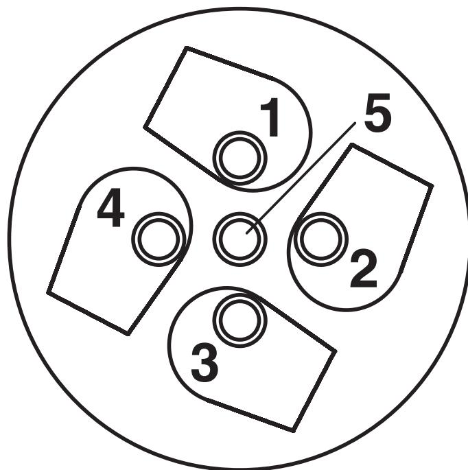
Cable connection side M12 (screw connection)
