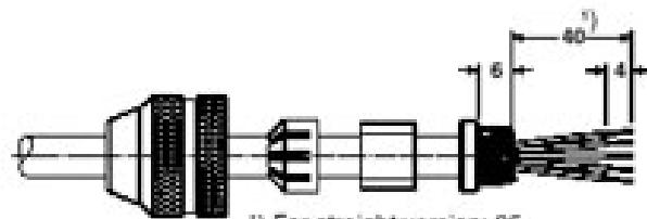
Strip conductor, widen shield and lay around the shielding ring, cut off projecting mesh.
