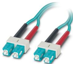
Assembled FO cable, zip cord cable, multi-mode fiberglass 50/125  $\mu\text{m}$ , OM3, plug: SC duplex/SC duplex, degree of protection: IP20, for installation in cable ducts or control cabinets, length: 2 m
