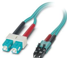
Assembled FO cable, zip cord cable, multi-mode fiberglass 50/125 µm, OM3, plug: LC/SC duplex, degree of protection: IP20, for installation in cable ducts or control cabinets, length: 2 m
