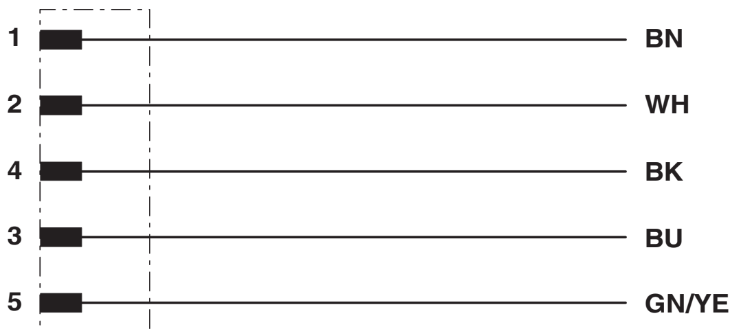
Contact assignment of the M12 plug
