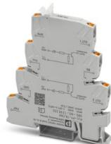
The inverter module with Push-in connection inverts the signals of ground switching NPN transistor outputs into positive switching PNP outputs, as well as signals from PNP into NPN switching signals.
