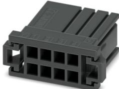
PCB connector, color: black, nominal current: 8 A, rated voltage (III/2): 160 V, contact surface: Sn, contact connection type: Socket, number of rows: 2, number of positions: 8, product range: DD31PC 2,2/.., pitch: 3.81 mm, connection method: Crimp connection, conductor/PCB connection direction: 0 °, locking clip: - without locking clip, plug-in system: CONNEXIS DD, locking: Snap-in locking, mounting method: Latching flange, type of packaging: packed in cardboard
