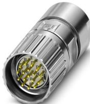
M23, Cable connector, series: M23 PRO, straight, shielded: yes, Screw locking mechanism, No. of pos.: 17, Direction of rotation: Standard, contact connection type: Pin, Solder connection, cable diameter range: 4 mm ... 8.5 mm, coding: N, Item is lead-free in accordance with RoHS II without Exemption 6c (Pb < 0.1 %)
