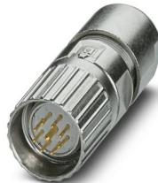
M23, Cable connector, series: M23 PRO, straight, shielded: yes, Screw locking mechanism, No. of pos.: 8+1, Direction of rotation: Standard, contact connection type: Pin, Solder connection, cable diameter range: 3 mm ... 15 mm, coding: N, Item is lead-free in accordance with RoHS II without Exemption 6c (Pb < 0.1 %)
