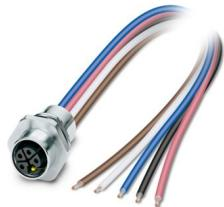
Device connector front mounting, Power, 5-position, Flush-type female connector, straight, M12-Standard, L-coding, on free cable end, Individual wires, cable length: 1 m, 2.50 mm<sup>2</sup>, PEX litz wire
