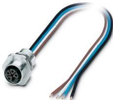
Device connector front mounting, Power, 4-position, Flush-type female connector, straight, M12-Standard, L-coding, on free cable end, Individual wires, cable length: 2 m, 2.50 mm<sup>2</sup>, PEX litz wire
