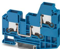
Feed-through terminal block, nom. voltage: 1000 V, nominal current: 57 A, number of connections: 3, number of positions: 1, connection method: Push-X-connection, Rated cross section: 10 mm<sup>2</sup>, cross section: 1.5 mm<sup>2</sup> - 16 mm<sup>2</sup>, mounting type: NS 35/7,5, NS 35/15, color: blue
