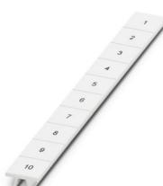
Zack marker strip, Strip, white, labeled, can be labeled with: CMS-P1-PLOTTER, Printed vertically: consecutive numbers 1 ... 10, 11 ... 20, etc. up to 91 ... 100, mounting type: latching, for terminal block width: 10.2 mm, Number of individual labels: 10, text field height: 10.5 mm, text field width: 10.15 mm
