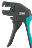
Stripping tool, for cables and conductors from 0.02 - 10 mm<sup>2</sup>, self-adjusting, stripping length of up to 18 mm, cutting capacity of up to 10 mm<sup>2</sup> stranded/1.5 mm<sup>2</sup> solid, replaceable stripping blade
