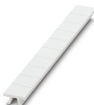
Zack marker strip, can be ordered: Strip, white, labeled according to customer specifications, mounting type: snap into tall marker groove, for terminal block width: 10.2 mm, Number of individual labels: 10, text field height: 10.5 mm, text field width: 10.15 mm
