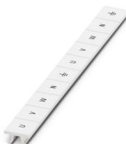
Marker for terminal blocks, Strip, white, labeled, can be labeled with: CMS-P1-PLOTTER, horizontal: U, V, W, N, GND, U, V, W, N, GND, mounting type: latching, for terminal block width: 10.2 mm, Number of individual labels: 10, text field height: 10.5 mm, text field width: 10.15 mm
