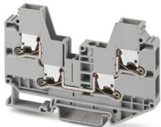
Feed-through terminal block, nom. voltage: 1000 V, nominal current: 41 A, number of connections: 4, number of positions: 1, connection method: Push-X-connection, Rated cross section: 6 mm<sup>2</sup>, cross section: 0.5 mm<sup>2</sup> - 10 mm<sup>2</sup>, mounting type: NS 35/7,5, NS 35/15, color: gray
