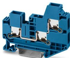
Feed-through terminal block, nom. voltage: 1000 V, nominal current: 41 A, number of connections: 3, number of positions: 1, connection method: Push-X-connection, Rated cross section: 6 mm<sup>2</sup>, cross section: 0.5 mm<sup>2</sup> - 10 mm<sup>2</sup>, mounting type: NS 35/7,5, NS 35/15, color: blue
