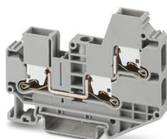
Feed-through terminal block, nom. voltage: 1000 V, nominal current: 41 A, number of connections: 3, number of positions: 1, connection method: Push-X-connection, Rated cross section: 6 mm<sup>2</sup>, cross section: 0.5 mm<sup>2</sup> - 10 mm<sup>2</sup>, mounting type: NS 35/7,5, NS 35/15, color: gray
