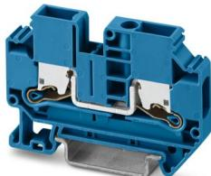
Feed-through terminal block, nom. voltage: 1000 V, nominal current: 41 A, number of connections: 2, number of positions: 1, connection method: Push-X-connection, Rated cross section: 6 mm<sup>2</sup>, cross section: 0.5 mm<sup>2</sup> - 10 mm<sup>2</sup>, mounting type: NS 35/7,5, NS 35/15, color: blue
