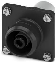
Connector, Range of articles: BPC, color: black, number of positions: 1, min. conductor cross-section: 95 mm<sup>2</sup>, max. conductor cross-section: 120 mm<sup>2</sup>, rated voltage: 1500, rated current: 350 A, Connection method: Crimp
