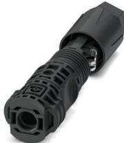
Connector, Range of articles: SUNCLIX, color: black, number of positions: 1, min. conductor cross-section: 6 mm<sup>2</sup>, max. conductor cross-section: 16 mm<sup>2</sup>, rated voltage: 1500 V DC, rated current: 60 A, Connection method: Spring-cage, min. cable diameter: 5.5 mm, max. cable diameter: 10 mm
