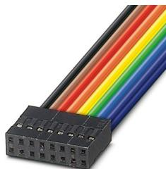
Power connector for DIN rail bus connector with 16 free cable ends with a cross section of 0.25 mm<sup>2</sup>, 500 mm long, female contacts
