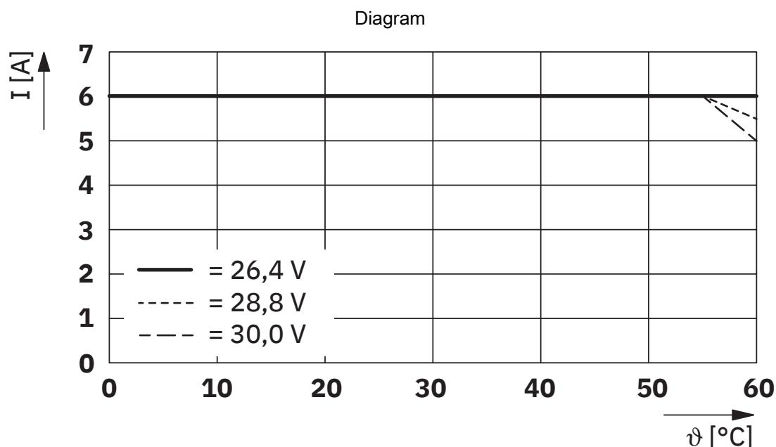
Max. switching current of the PLC-R...24DC/21 and PLC-R...24DC/21EX modules in combination with PLC-V8R...
