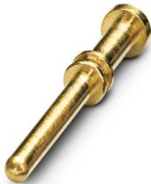
Crimp contact, Pin, turned, contact diameter: 2 mm, connection cross section: 0.25 mm<sup>2</sup> ... 2.5 mm<sup>2</sup>, contact material: CuZn, Item is lead-free in accordance with RoHS II without Exemption 6c (Pb < 0.1 %)
