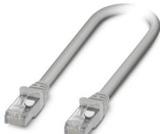
Patch cable, degree of protection: IP20, cable length: 20 m, number of positions: 8, CAT5, connection method: Pierce connection, connection cross section: AWG 26- 26, cable outlet: straight, Ethernet, 2x2xAWG26/7, S/UTP, gray
