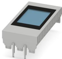
DIN rail housing, 10U upper part, integrated 2.4" resistive touch display, resolution: 320 x 240 Pixel(s), interface: 4-wire SPI half duplex, Housing cover, width: 56.88 mm, height: 109.8 mm, depth: 29.5 mm
