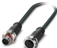
Sensor/actuator cable, 4-position, PUR halogen-free, black-gray RAL 7021, shielded (Advanced Shielding Technology), Plug straight M12 Push Pull, coding: A, on Socket straight M12 Push Pull, coding: A, cable length: 1.5 m
