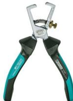
Stripping pliers, for removing the sheath from cables up to 5 mm in diameter, for stripping conductors with a cross section of up to 10 mm<sup>2</sup>, scale for measuring the stripping length; VDE-tested. Type of packaging: with bracket for sales display (backcard)
