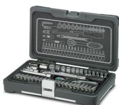
**1/4" socket set**, 47-piece, 1/4" reversible ratchet, 48 teeth with fast locking system, 50 mm and 100 mm 1/4" extensions, 1/4" screwdriver handle, 150 mm 1/4" flexible extension, 1/4" Cardan joint, 1/4" T-handle
