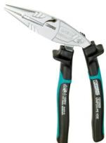
**Needle-nose pliers**, angled design, with opening spring and locking device, finely notched grip area, stripping possible for 1.5 mm<sup>2</sup> and 2.5 mm<sup>2</sup>, integrated M8 - M10 ring wrench, VDE 1000 V AC/1500 V DC tested
