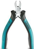
Electronic diagonal cutter, round head, without chamfer, with opening spring, mirror-polished and oiled, 2-component grip, cutting capacity: soft 0.2 - 2.0 mm; medium hard 1.2 mm; hard 0.5 mm diameter
