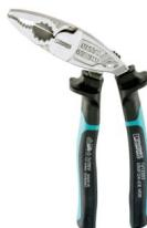
**Combination pliers**, angled design, with opening spring and locking device, cross-notched grip area, integrated M8 - M10 ring wrench, VDE 1000 V AC/1500 V DC tested
