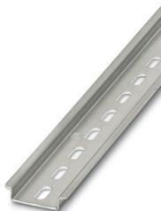
DIN rail perforated, acc. to EN 60715, length: 500 mm, material: Steel, galvanized, passivated with a thick layer, mounting type: Standard profile, color: silver, Current dimensional tolerances: Profile tolerance due to burr/sharp edges =  $\pm 0.5$  mm, Initial dimension =  $\pm 0.5$  mm, Hole pattern =  $\pm 0.5$  mm, Hole position =  $\pm 0.5$  mm, Minimum rail length: Unperforated: > 20 mm, Perforated: > 100 mm, Last punching at Phoenix Contact: < 1750 mm
