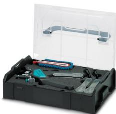
Tool for processing ferrules according to DIN 46228-4, 0.5 mm<sup>2</sup> to 2.5 mm<sup>2</sup>, equipped with pressure lock, cutting, stripping, twisting, and crimping unit, with three magazines including a strip each of ferrules from 0.5 mm<sup>2</sup> ... 2.5 mm<sup>2</sup>, packaged in a robust plastic case
