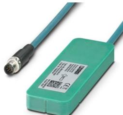
Sensor for measuring loads on the rotor blade of wind turbine generators. Robust (can be stood on). With magnetic shielding. Cable resistance compensation thanks to 6-wire connection technology.
