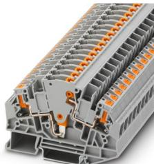
Test disconnect terminal block, nom. voltage: 1000 V, nominal current: 30 A, connection method: Push-in connection, Rated cross section: 6 mm<sup>2</sup>, cross section: 0.5 mm<sup>2</sup> - 6 mm<sup>2</sup>, color: gray
