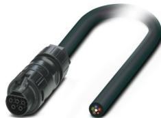
Connecting cable, Range of articles: PRC 35, color: black, number of positions: 5, max. conductor cross-section: 2.5 mm<sup>2</sup>, rated voltage: 690 V AC, rated current: 32 A, Connection method: Screw connection, This item is also available with other cable lengths. For your specific requirements, please contact your local PHOENIX CONTACT subsidiary.
