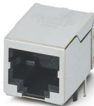
Modular RJ45 PCB connectors, 1x1 single-port, connection direction of the connector to the PCB: 90 °, Tab down, Shielded, number of positions: 8, 10 Gbps, PoE++, THT, Wave, type of packaging: Tray
